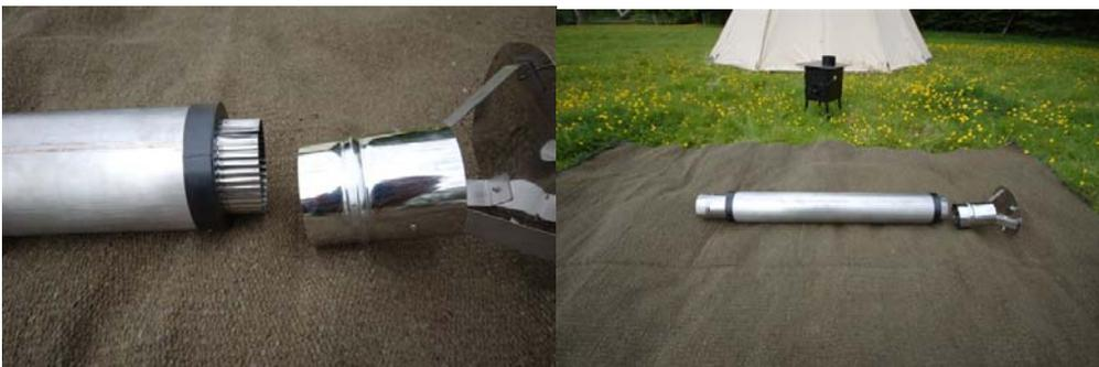
Start with the top piece with the double skin heat protector and make sure you have correct end with the cap so the sheath doesn't slip down when the piece is vertical. This then sets you up for the rest of the build.
