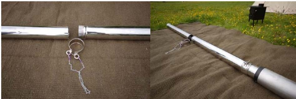
On the next joint use the clamp with the securing chain and attach in the same way
